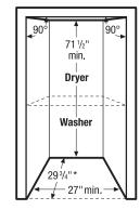
Stacked Units in Recessed or Closet Installation For detailed stacked installation, refer to instructions included with Stacking Kit or on web. Note: Stacked installatic
