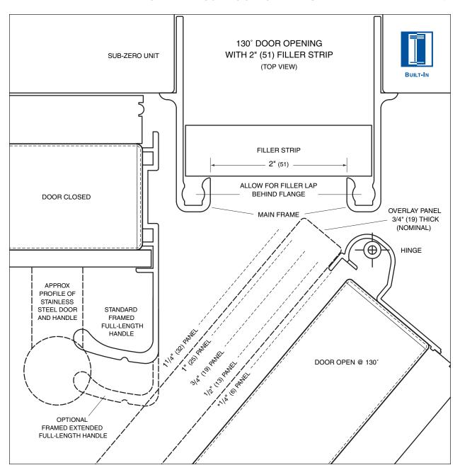
The full-scale illustration above shows the panel and handle profile of a 130° door opening with 2" (51) filler strip for framed applications.
