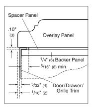
► Three panel assembly—cross section
