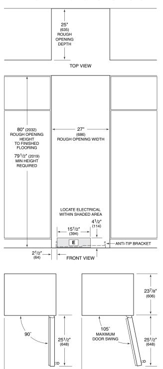
NOTE: Door swing clearances are based on stainless steel door and handle dimensions.
