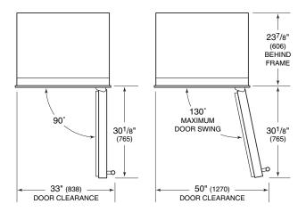
NOTE: Door swing clearances are based on stainless steel door and handle dimensions.
