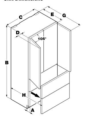
Overall height can be increased on HC 20 and HCS 20 units by 1-1/2" (40 mm) by adjusting the roller base.
