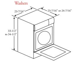
**Depth with Door Open** W600 & W640 — 36-3/8" W620 & W660 — 42-3/8"
