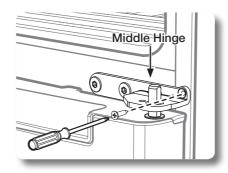
2. After removing one screw and two bolts, remove the Middle Hinge. (Unscrew the screws with the screwdriver(+) and hex bolts with the 3/16inch hex wrench.)
