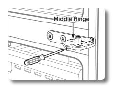
2. After removing one screw and two hex bolts, remove the Middle Hinges. (Unscrew the two hex bolts with the 3/16inch hex wrench.)
