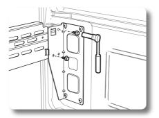
4. With the 7/16inch wrench, remove two bolts connecting the rail with the door.
