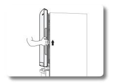
6. Remove the fridge door by lifting it upward. Be careful not to drop and scratch the fridge door.
