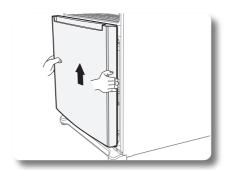
Remove the Freezer door by lifting it upward.
