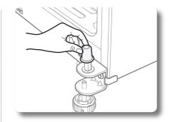
5. Remove the Cap on the Bottom Hinge.
