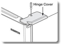
1. After removing the screw, remove 2. Disconnect electric wire on the the upper Hinge Cover.
