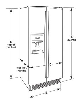
Dimensions "D" and "E" include rollers extended 3/4".
