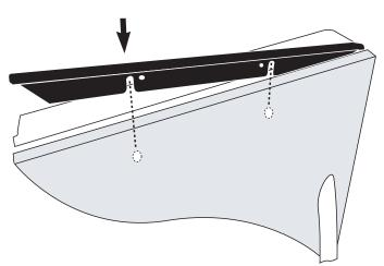
8. Fully seated top trim completely covers clips of side trim and is close to flush with the top of the door.
