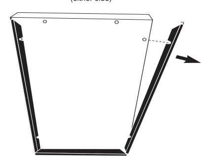
3. Slide decorator panel under edges of bottom and side trim pieces. Reinstall side trim, assuring the side trim clip locates to the inside corner of the bottom trim.
