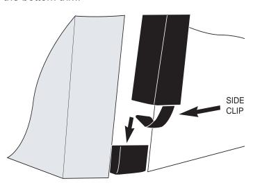
4. Rotate side trim to seat into the decorator panel groove.
