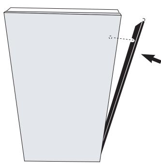
5. Align the upper locking trim with the clips on top of the side trim.
