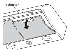
To remove filters: Pull the deflector down. Push the handles toward the back of the hood and pull down.
