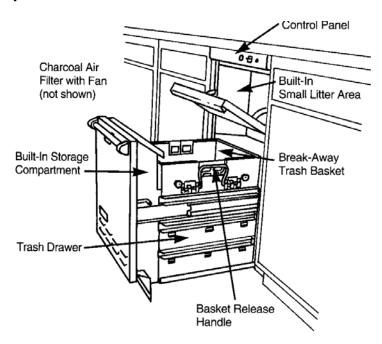
Your compactor has a built-in interlock and will not operate unless you have:
