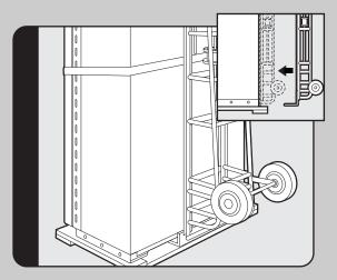
Slip cart between unit and skid. Remove unit from skid. Note: Use excess packaging to protect decorative trim; also, verify that leveling legs are up (0" adjustment).
