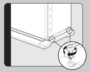
Remove shipping brackets from skid by removing 4 bolts (2 on each side) with a 1/2" deep-well socket wench and a pair of pliers. Note: Tilting unit is not required to remove shipping brackets.
