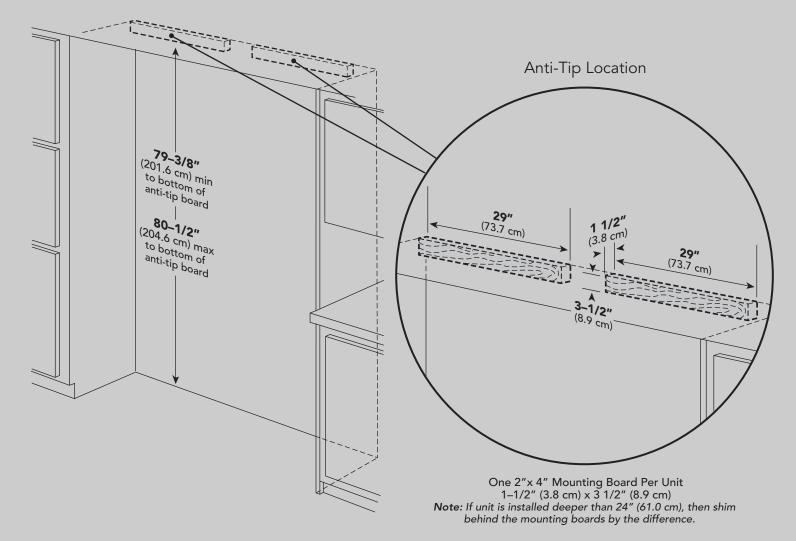
Bottom of anti-tip board is 3–7/8" (9.8 cm) below opening height. Note: Top of unit must be placed firmly under anti-tip board.
