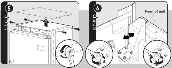
Remove four side screws and remove unit top.
