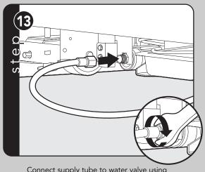
Connect supply tube to water valve using a 1/2" wrench. Note: DO NOT overtighten.
