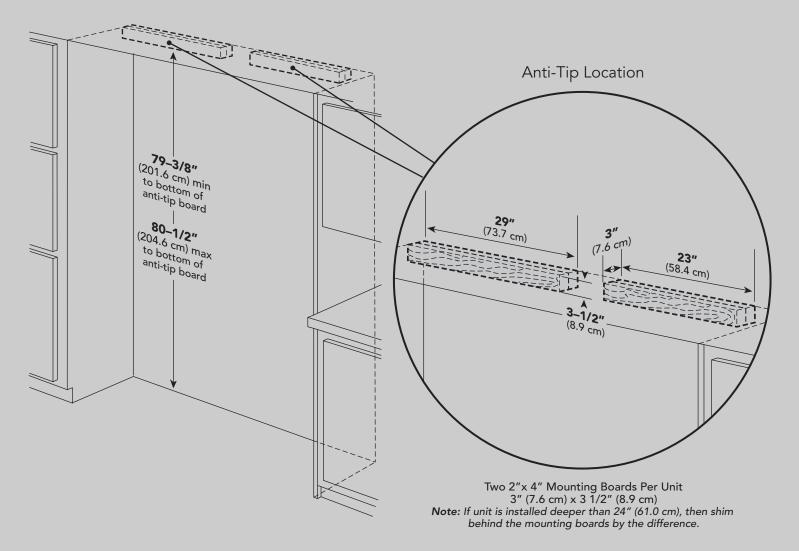
Bottom of anti-tip board is 3–7/8" (9.8 cm) below opening height. Note: Top of unit must be placed firmly under anti-tip board.
