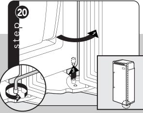
Open refrigerator door so door stop and shoulder screw are accessible. Note: Shoulder screw should be in 110P door opening position.
