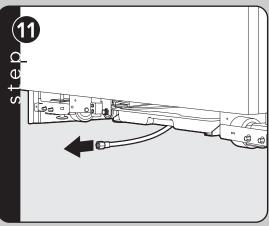
Pull supply tubing forward under unit. Note: DO NOT use plastic water lines.
