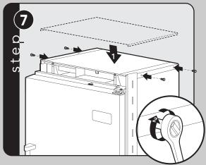
Replace unit top. Replace four side screws.
