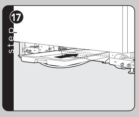
Verify that drain pan is installed and aligned.
