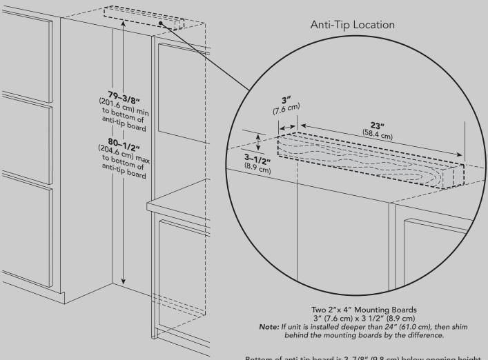
Bottom of anti-tip board is 3–7/8" (9.8 cm) below opening height. Note: Top of unit must be placed firmly under anti-tip board.
