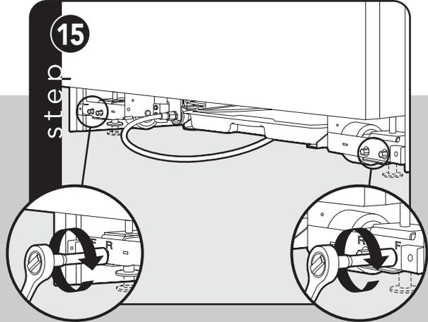
Lift unit off rollers to desired height and level unit using a 5/16" head wrench.
