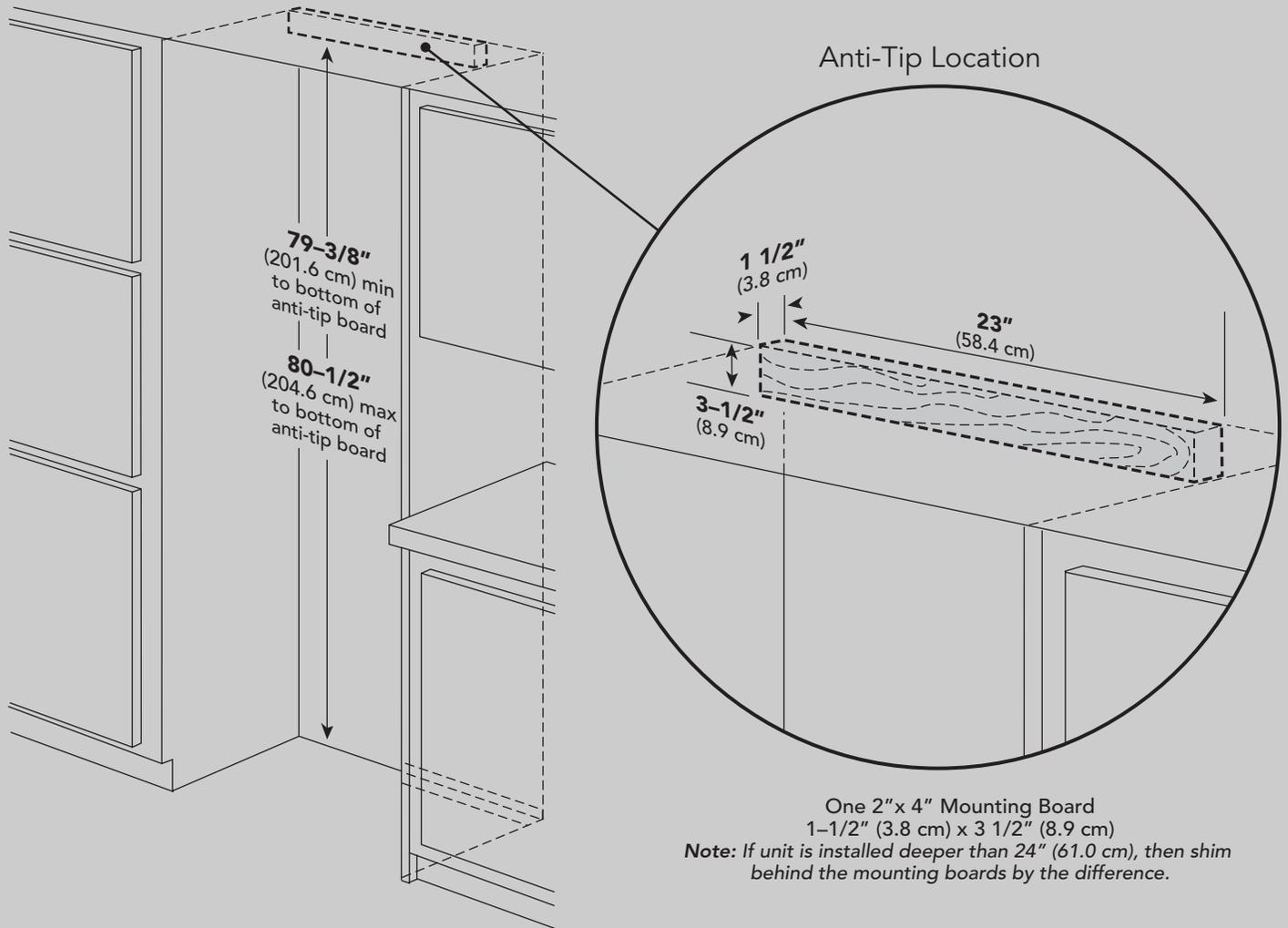
Bottom of anti-tip board is 3-7/8" (9.8 cm) below opening height.
