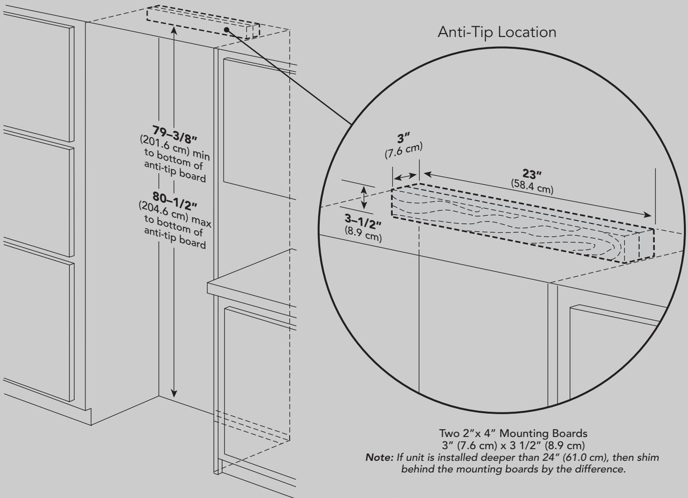
Bottom of anti-tip board is 3-7/8" (9.8 cm) below opening height.
