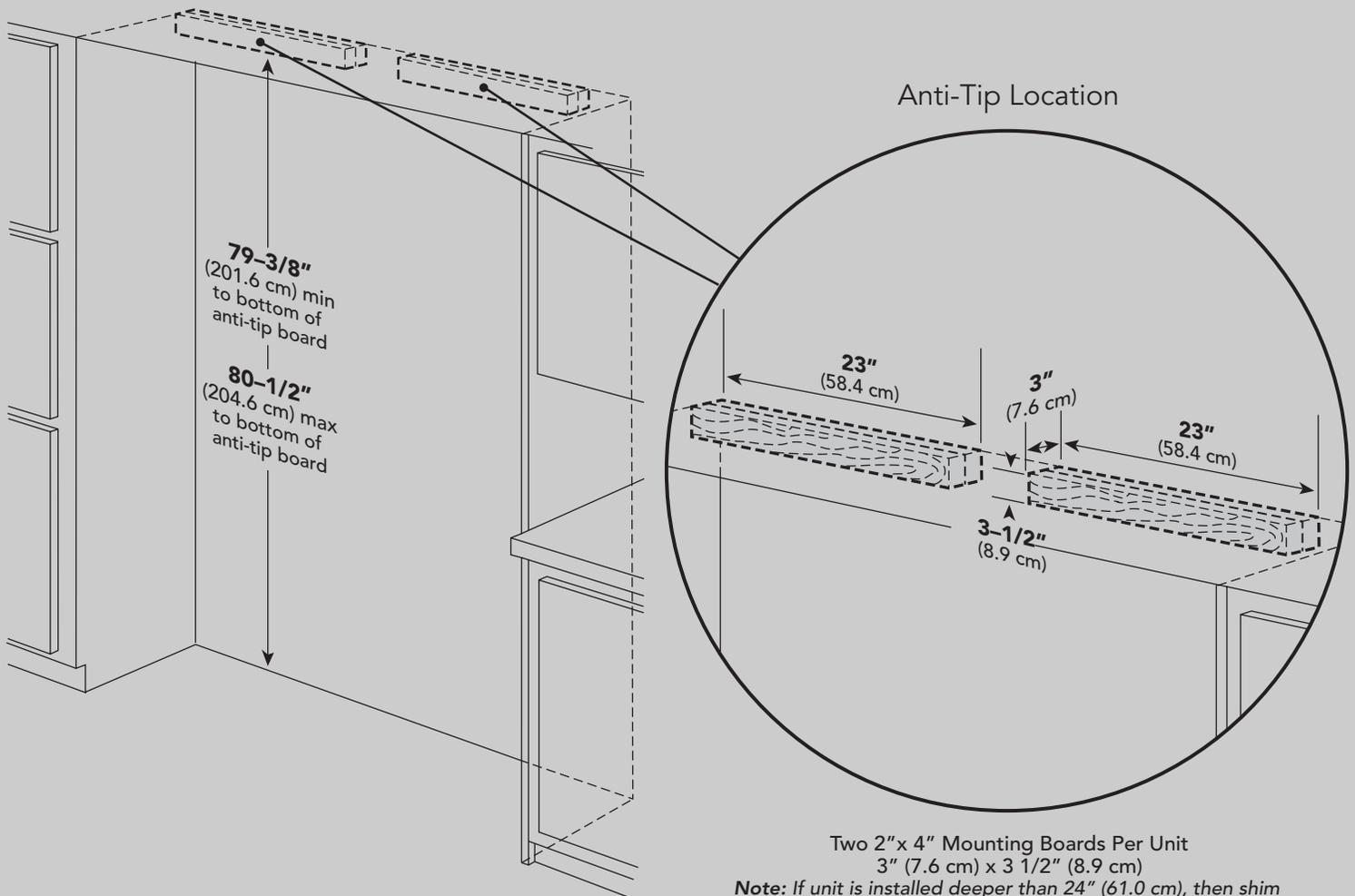
**Note:** If unit is installed deeper than 24" (61.0 cm), then shim behind the anti-tip bracket by the difference.
