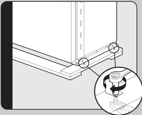
Remove shipping brackets from skid by removing 4 bolts (2 on each side) with a 1/2" deep-well socket wrench and a pair of pliers.
