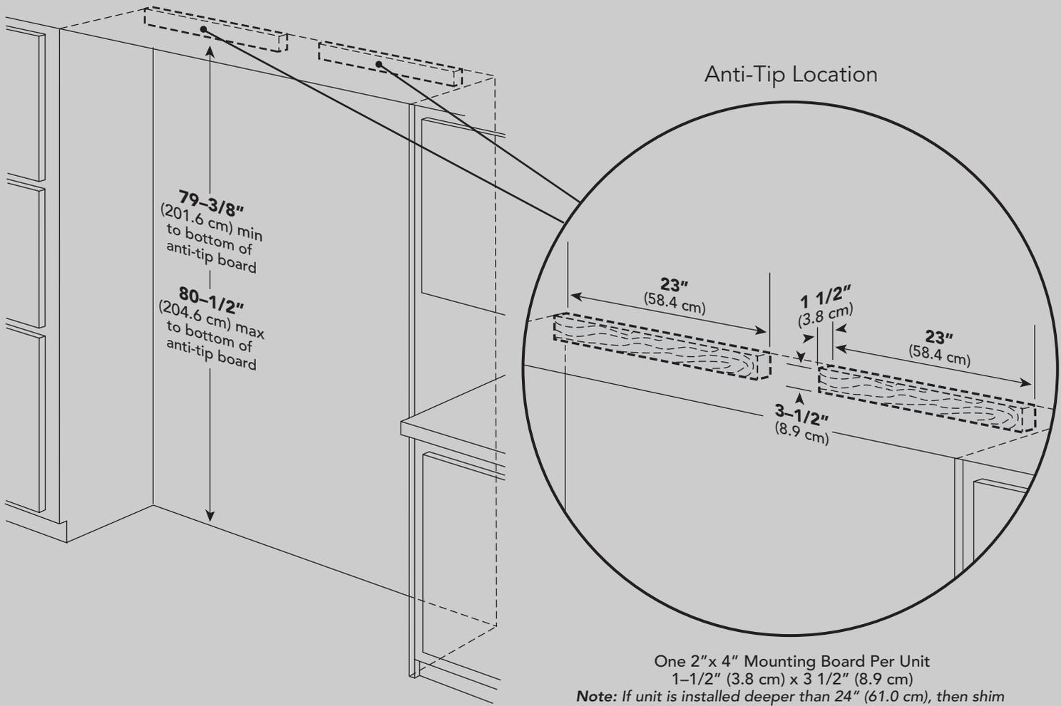
Bottom of anti-tip board is 3-7/8" (9.8 cm) below opening height.
