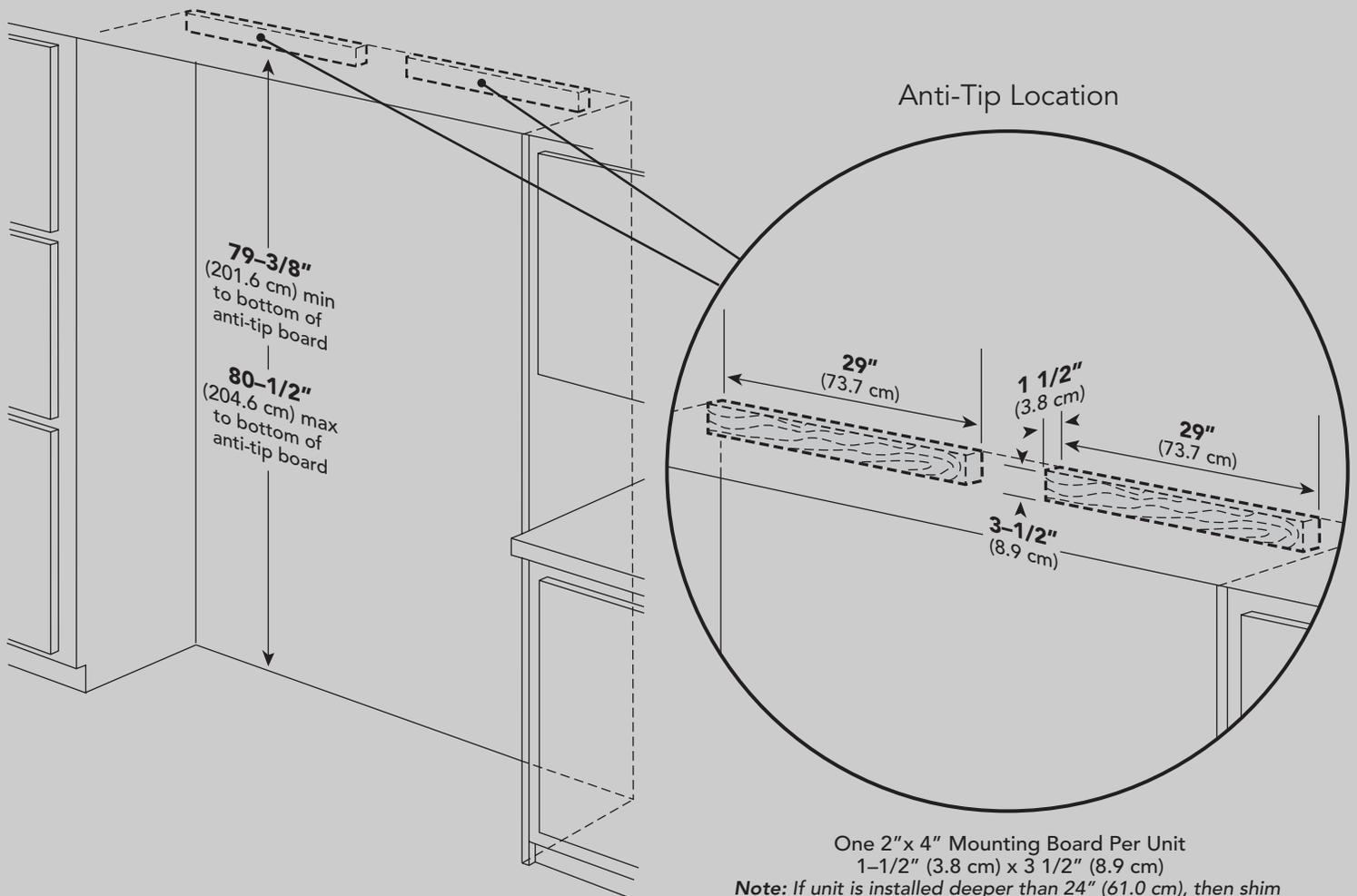
**Note:** If unit is installed deeper than 24" (61.0 cm), then shim behind the mounting boards by the difference.
