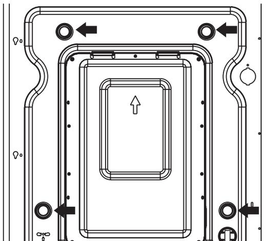
2. Unscrew the 4 bolts with the wrench supplied. Keep the 4 bolts and wrench for future use.
