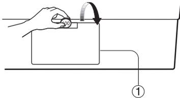
2. Unplug the hose cap (2) and drain the water into a shallow bowl or some old towels. When the water flow stops, turn the pump filter (3) counterclockwise to remove it.
