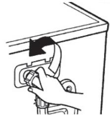
3. Pull the inlet filter out. Remove the dirt from the inlet filter with a brush.
