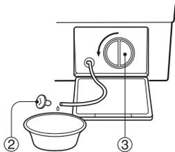
3. Remove any debris that is in the pump filter. (3). Once clean, replace the pump filter by turning it clockwise. Plug the drain hose with the hose cap and snap the hose into its holder. Close the drain pump cover.
