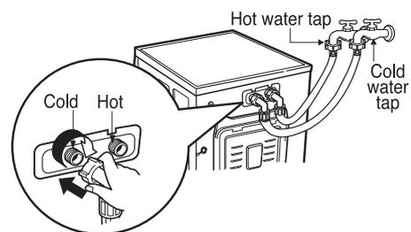
valve on the wall and that cold is connected to cold. The hot water hose has a red stripe, the cold has a blue stripe.
