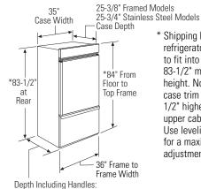
\* Shipping height. The refrigerator can be adjusted to fit into a cutout that is 83-1/2" min. to 84-1/2" max. height. Note that the top case trim at the front is 1/2" higher and will overlap upper cabinetry or soffit. Use leveling legs and wheels for a maximum 1" height adjustment.
