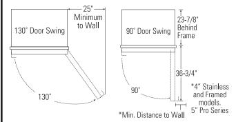
Allow 25" minimum clearance for a full  $130^{\circ}$  door swing. Allow 15" for pan removal.
