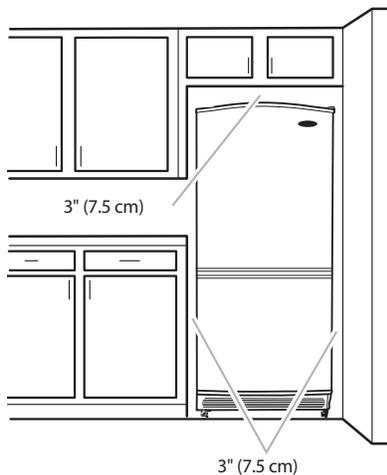
Allow at least 3 in. (7.5 cm) of air space at the top and on both sides of the freezer and 1 in. (2.5 cm) between the back of the freezer and the wall. If the freezer is to be against a wall, leave extra space on the hinge side so the door can open wider.
