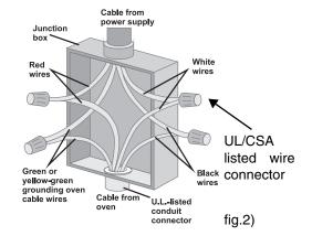
Connect to a 20A fuse or circuit breaker. Connect to copper wire only, or, if connecting to aluminum house wire, use UL-listed or CSA-approved connectors, which are suitable for joining aluminum with copper wires.
