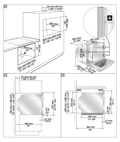
**IMPORTANT:** This appliance must be integrated in any cabinets made of material which is heat resistantup to temperatures of 194°F-90°C.
