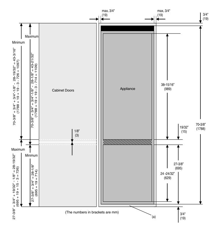
The gap between refrigerator and freezer door must lie within the crosshatched area.
