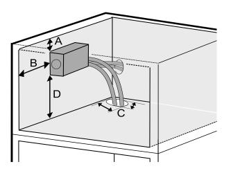
Maintain the dimensions shown in Fig. so that the filter can be replaced and the cover can be removed.
