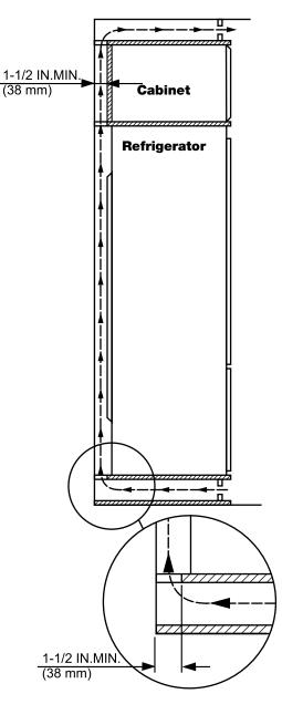
A minimum space of 1 1/2" is required when a cabinet is built above and/or underneath.
