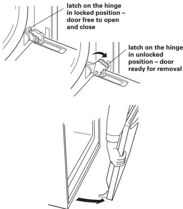
**2.** Completely open oven door. In both back corners of the door you will see door latches in the locked position. Rotate both latches forward to the unlocked position.
