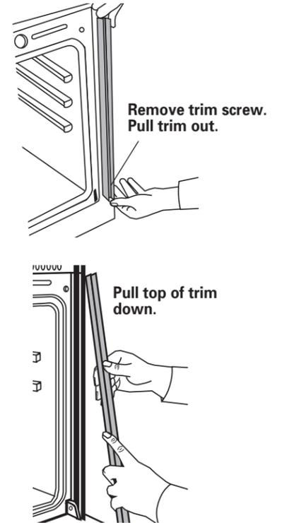
**3.** Remove trim screws attaching right and left side trim to oven. Grasp the bottom end of trim and pull away from oven. Slide top end of trim downward to remove trim from oven. Take care not to scratch other surfaces with ends of trim. Set trim and screws aside on protected surface.
