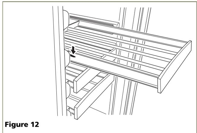
3. Press the left rack release lever (**Figure 12**) down, and at the same time, lift the corresponding right rack release lever up, and pull the rack out until it is free of the tracks and the cabinet.
