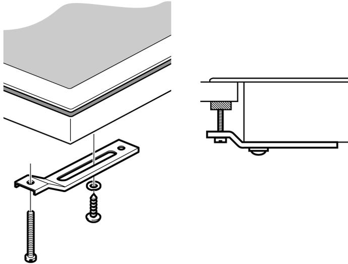
The cooktop should be secured to the countertop using the hold-down brackets provided.
