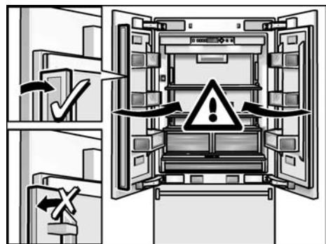
**Care should be taken when closing the door. The appliance could become damaged!**
