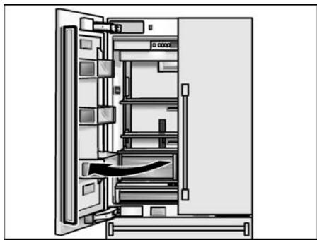
The 3-door variant allows for the left refrigerator compartment door to be opened without first having to open the right door.
