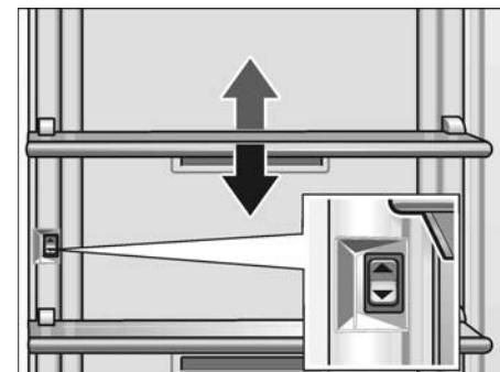
The height of this shelf can be adjusted when it is loaded.
