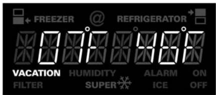
The **VACATION** symbol is displayed. Instead of the required temperature, the presetting temperature is displayed.
