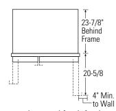
Allow minimum clearances for freezer door and fresh food door for a full 130° door swing and to allow for pan removal.
