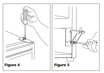
Remove bottom hinge from cabinet (two screws). See Figure 5. Remove screws on opposite side of cabinet (Figure 6). Note that there may be a nut behind one or both screws on either side.
