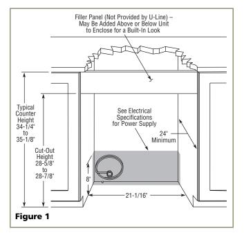
Follow the cut-out drawing in **Figure 1**. The 21-1/16" width allows 1/4" for ease in installation and removal of the unit. 24" is the counter depth in most installations. The unit is 24" deep including the door and handle (see **Figure 2**).
