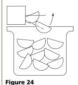
arm into an upright and locked position (see **Figure 24**). While the bin arm is locked, the unit will maintain temperature for ice storage.
