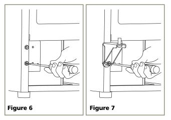
Install hinge on opposite side, bottom of cabinet. See Figure 7. Replace nut on back side where installed. Align hinge outer edge with cabinet before tightening screws.
