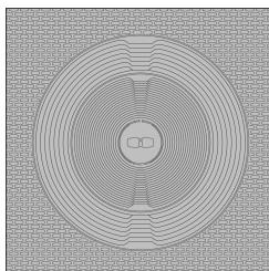
The dual element comprises two cooking zones: an inner one and an outer one.
