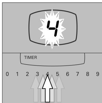
2. Within 5 seconds, slide your finger across the slider panel until the desired heat setting appears in the element display.
