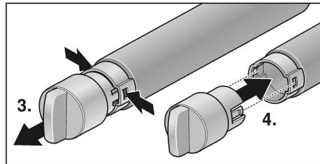
3. Remove the cap from the used filter.
