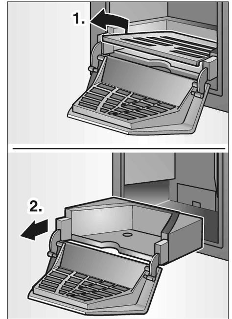
Spilled water collects in the water collecting tray of the pitcher holder. The water collecting tray can be emptied and cleaned by pulling out the pitcher holder.
