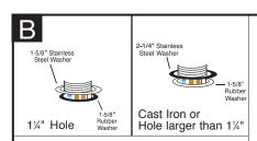
Make sure to use rubber washer to ensure proper seal.
