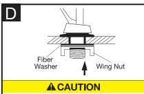
Property Damage: Do not over tighten the plastic wing nut.
