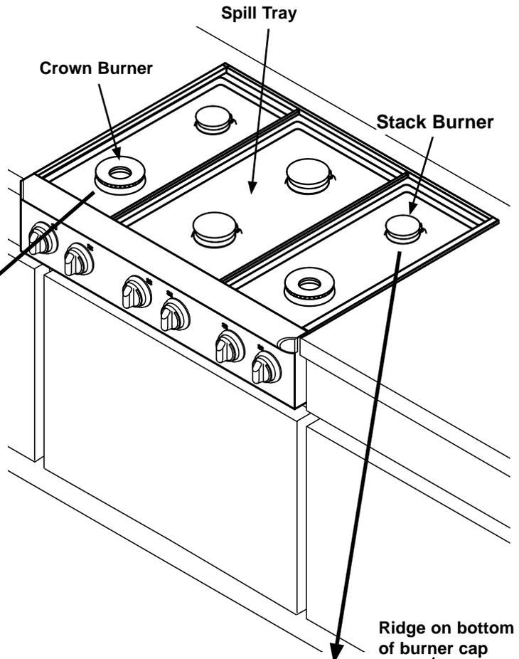
**STEP 3:** Install burner cap. Ridge on cap must surround top of ring.
