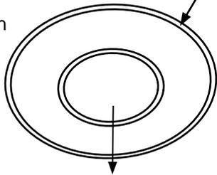
**STEP 2:** Install burner ring. Line up ring tabs with head slots. Twist back and forth to assure proper seating.
