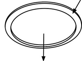
**STEP 2:** Turn ring until it drops into place. Twist back and forth to assure proper seating.
