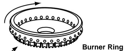
**STEP 1:** Put burner ring on top of the head.
