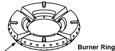
**STEP 1:** Install burner head. Put locating tap into keyed hole.
