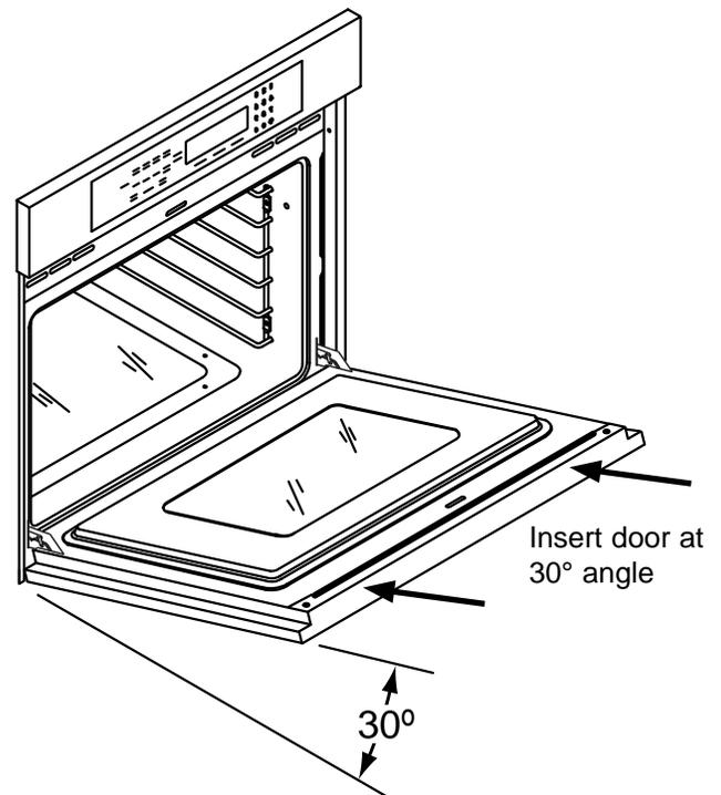
3. Lower the door to the fully opened position. Rotate both hinge catches toward the oven. Open and close the door slowly and completely to ensure that it is properly installed.
