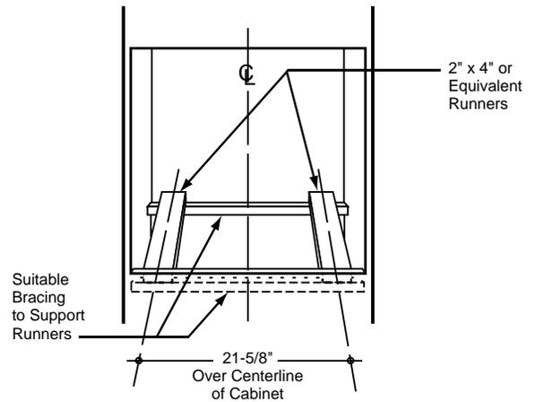
If the cabinet does not have a solid bottom, two braces or runners must be installed to support the weight of the oven. For single ovens, the runners and braces must support 150 lbs.
