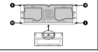
3 Attach the exhaust adaptor to the rear mounting plate by sliding it into the guides at the top center of the plate on the wall side.
