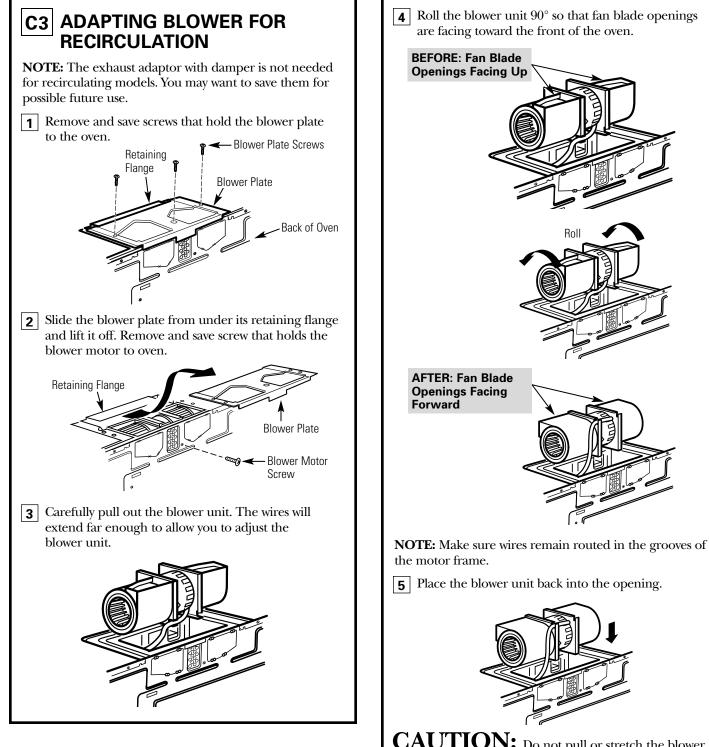
**CAUTION:** Do not pull or stretch the blower unit wiring. Make sure the wires are not pinched.
