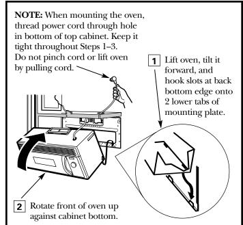
3 Insert a self-aligning screw through top center cabinet hole. Temporarily secure the oven by turning the screw at least **two full turns** after the threads have engaged. (It will be completely tightened later.) Be sure to keep power cord tight. Be careful not to pinch the cord, especially when mounting flush to bottom of cabinet.
