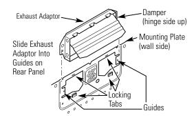
Push in securely until it is past the top locking tabs and in the lower locking tabs. Take care to assure the damper hinge is installed so that it is at the top and that the damper swings freely.
