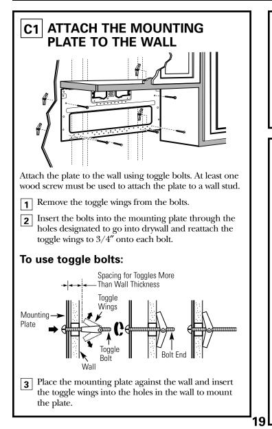
**NOTE:** Before tightening toggle bolts and wood screw, make sure the tabs on the mounting plate touch the bottom of the cabinet when pushed flush against the wall and that the plate is properly centered under the cabinet.
