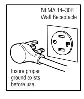
The wall outlet receptacle recommended for this appliance is NEMA # 14–30R and accepts the 4-prong grounded plug of this appliance. You should have the wall receptacle and circuit checked by a qualified electrician to make sure the receptacle is properly grounded.
