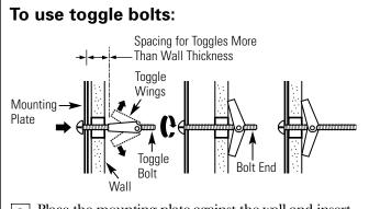
**3** Place the mounting plate against the wall and insert the toggle wings into the holes in the wall to mount the plate.
