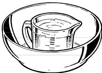
remains cool and only the water in the cup heats, then the dish is microwave-safe.
