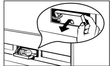
Reverse Step 2 and Step 3 to replace the grille, while making sure the grille is flush against the control panel.
