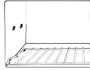
The metal shelf must be in place on the oven floor when using convection or combination cooking. The food is placed in a glass dish on a trivet for cooking during Combination Roast.
