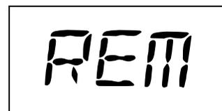
until you open the door or touch the CLEAR/OFF pad. The display will show “REM” until the oven door is opened or CLEAR/OFF is touched. The REMinder time may be displayed by touching the DELAY START pad. The time-of-day may be displayed by touching the CLOCK pad.
