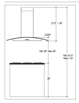
Minimum mount height between range top to hood bottom should be no less than 28".
