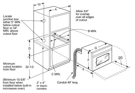
Suitable bracing to support runners (Must support 275 lbs.)
