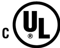
The UL Canadian listing mark consists of the circled UL symbol preceded by the letter “C,” as shown. This should appear on the oven’s rating plate along with the UL United States listing mark, which is the circled UL symbol above but not preceded by the letter “C.”
