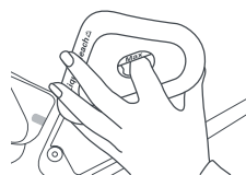
Fig.16 Removing the Bleach dispenser funnel
