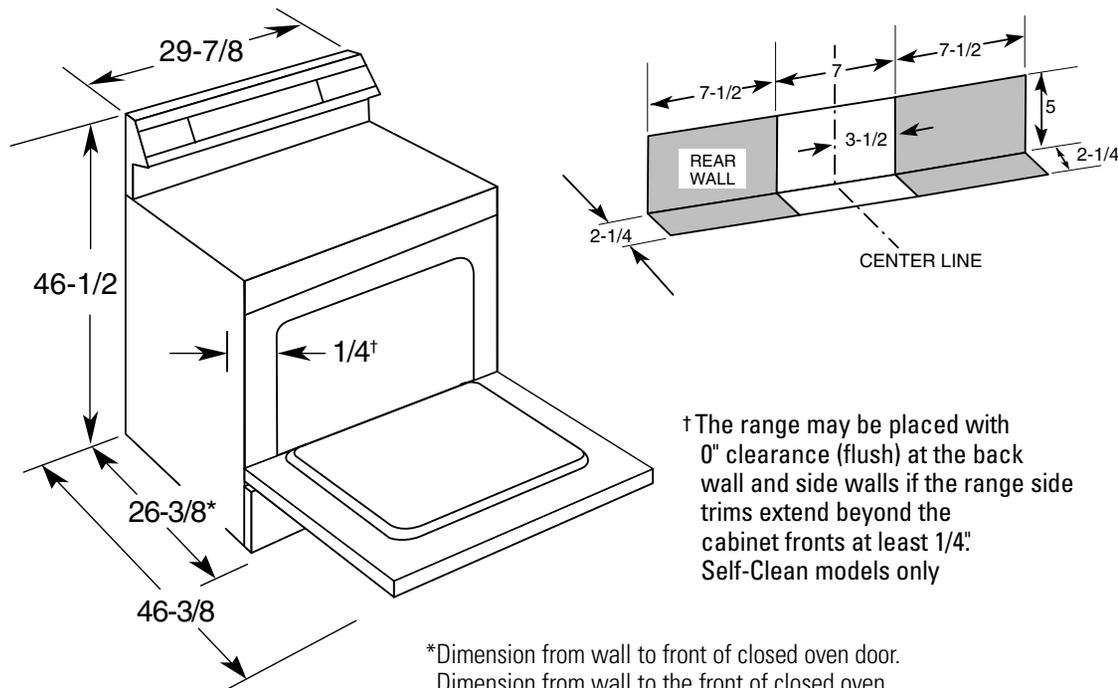
† The range may be placed with 0" clearance (flush) at the back wall and side walls if the range side trims extend beyond the cabinet fronts at least 1/4". Self-Clean models only
