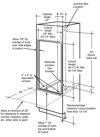
If the cabinet does not have a solid bottom, two braces or runners must be installed to support the weight of the oven. For double ovens, the runners and braces must support 275 lbs.
