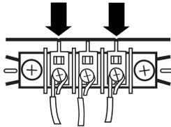
4. Tighten strain relief screw.
