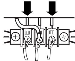
4. Tighten strain relief screws.
