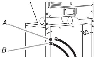
A. Cold water inlet valve (top)
