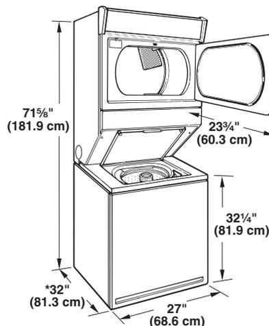
\*Most installations require a minimum 5½" (14 cm) clearance behind the dryer for the exhaust vent with elbow. See “Venting Requirements.”
