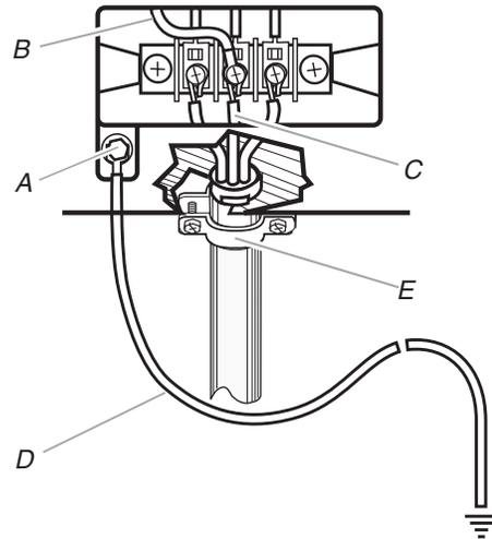
A. External ground conductor screw
