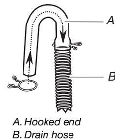
2. Put hooked end of drain hose into laundry tub or standpipe. Rotate hook to eliminate kinks.
