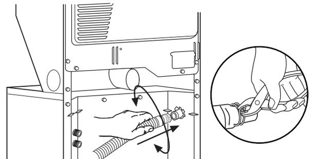
5. Place clamp over the area marked "CLAMP." Release clamp.
