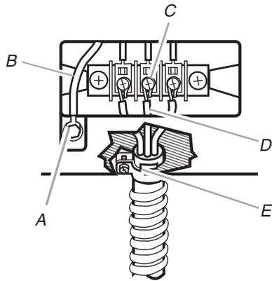
A. External ground conductor screw
