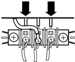
5. Tighten strain relief screw.
