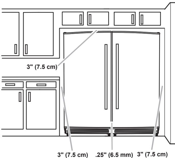
Allow at least 3 in. (7.5 cm) of air space at the top and on both sides of the appliances with 1/4 in. (6.5 mm) between the freezer and refrigerator. Allow 1 in. (2.5 cm) between the back of the appliances and the wall. If the appliances are to be against a side wall, leave extra space on the hinge sides so the door can open wider.
