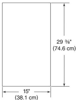
Panel should be a minimum of 1/2" (13 mm) thick.
