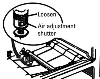
The shutter for the bottom (oven) burner is near the back wall behind the storage drawer or kick panel. Remove the drawer or panel. See the *Care and cleaning of the range* section.
