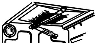
The flames for the top (broil) burner should be steady with approximately 1" blue cones and should not extend out over the edges of the burner baffle.
