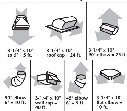
If the existing vent is round, a rectangular-to-round adapter must be used and a minimum 3" (7.6 cm) clearance must exist between the top of the microwave oven and the rectangular to round transition piece so that the damper can open freely and fully.
