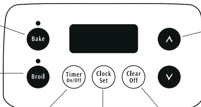
**UP and DOWN ARROW PADS**— Used along with the function pads to select oven temperature, time of day, clean time and minute timer.
