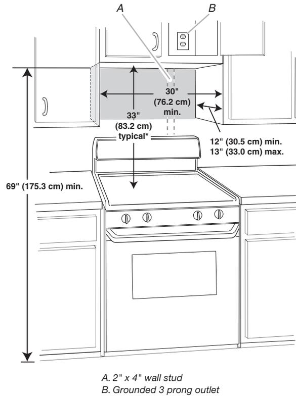
**NOTE:** The grounded 3 prong outlet must be inside the upper cabinet.
