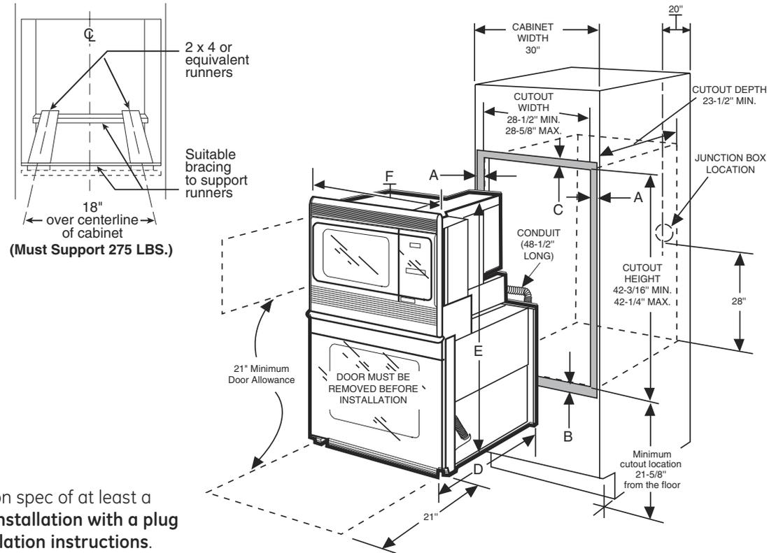
MOST 30" WALL CABINETS CAN BE USED WITH THIS UNIT. THE OPENING BETWEEN THE INSIDE WALLS MUST BE AT LEAST 28-1/2" WIDE.
