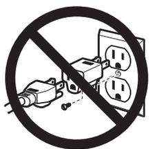
Do not use an adapter plug to connect the refrigerator to a 2-prong outlet.
