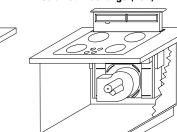
**Note:** Telescopic downdraft vents are not recommended to be installed with cooktops that are flush mounted.
