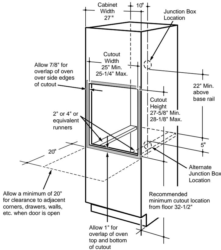
If the cabinet does not have a solid bottom, two braces or runners must be installed to support the weight of the oven. For single ovens, the runners and braces must support 150 lbs.
