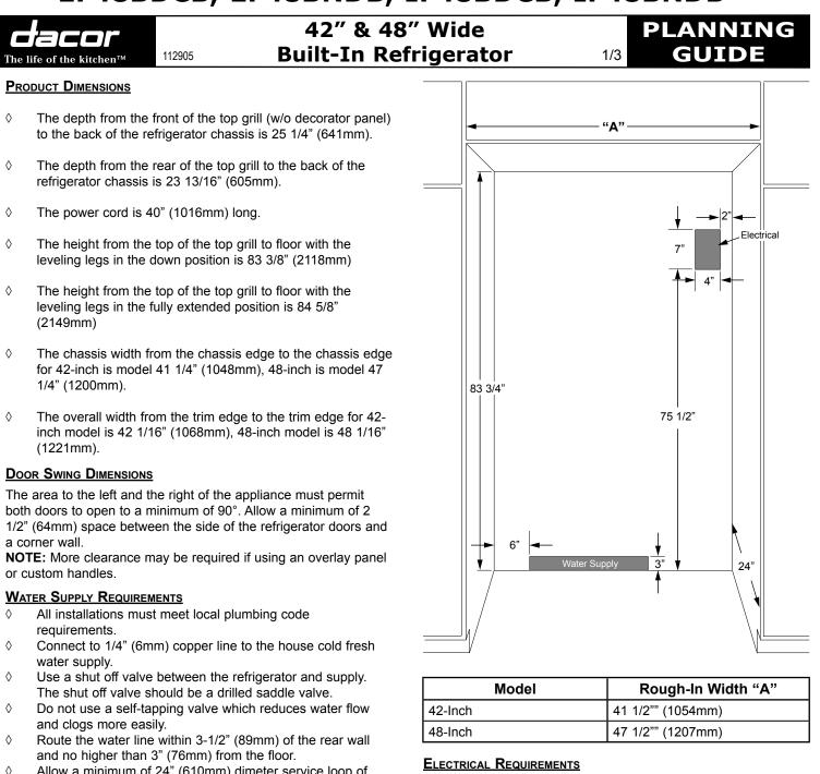
Allow a minimum of 24" (610mm) dimeter service loop of copper tubing outside the wall or floor for easy connection to the water supply.
