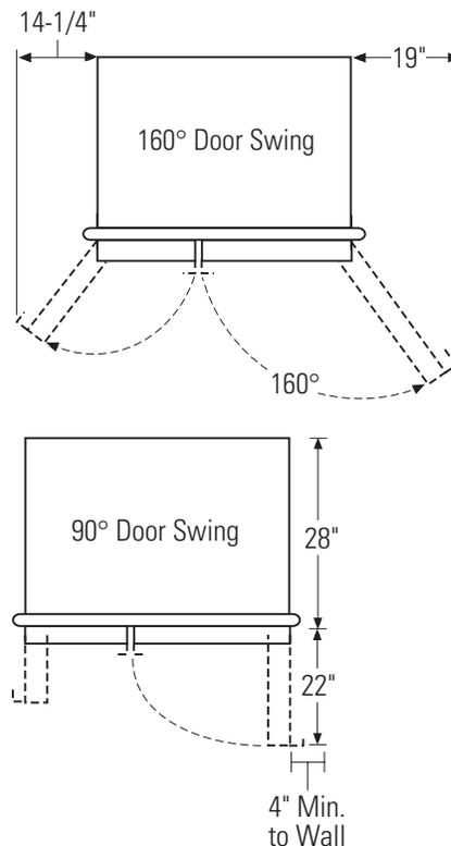
Allow 19" minimum clearance on the fresh food side for a full 160° door swing and pan removal. Allow 14-1/4" clearance on the freezer side for removal of ice bin.
